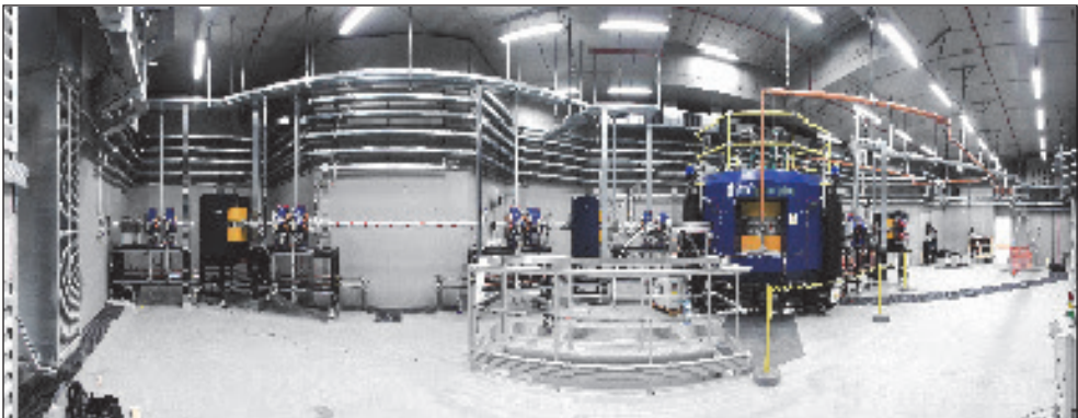
Fig. 6: The SPES radioactive ion beam facility, presently under construction at the Legnaro National Laboratories of INFN. The production cyclotron is visible (blue structure) on the right of the figure.
